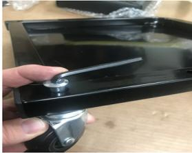
3. Install right and left upright brackets using 4 60mm bolts with 1 washer, and 1 nut each bolt using a 14mm wrench.
